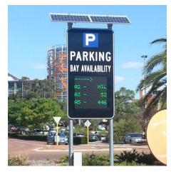
AD306 Car Parking Guidance Signs and Monitoring Systems provide high quality electronic LED display and vehicle detection system to inform motorists of car parking status and bay availability. Entry and exit may be monitored by ground loops and a central control system that tracks car parking status and displays the appropriate messages to the electronic displays. This type of system minimises traffic congestion and is also able to redirect some of the traffic flow to less congested areas.
